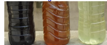
Dark leachate biologically decolourised without any chemical usage at Bentong LTP
